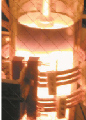
CVD system for SiC (HTC3100), supplied to National Institute of Advanced Industrial Science and Technology
