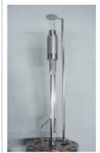
ECR Radical Cell adopts a unique mechanism to enable extremely highdensity plasma production. The ion removal mechanism (magnetic field system) provided at the top of the cell allows ion removal.
