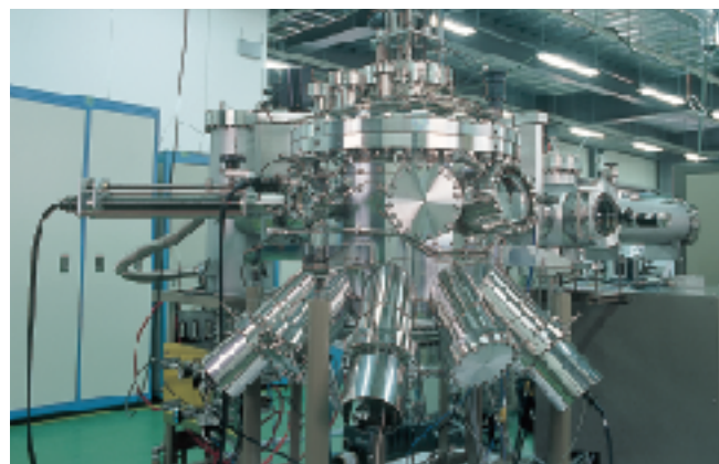
MBE system (RC6100) supplied to National Institute of Advanced Industrial Science and Technology
