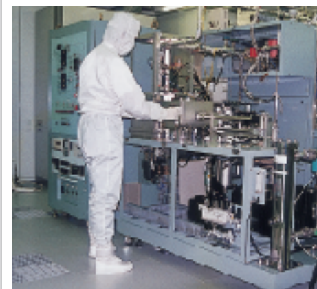
Liquid delivery MOCVD system (MPC6100) supplied to Nara Institute of Science and Technology
